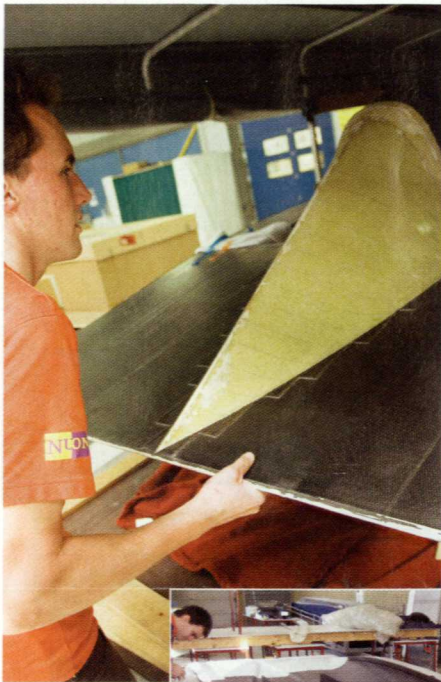
Above: The car's all-carbon top shell with integral aramid-skinned canopy is removed from the curing oven.
